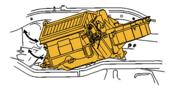
Refer to SI 2000 to obtain the service procedure for correctly removing and installing the HVAC module. Failure to do could result in damage to the HVAC module.
