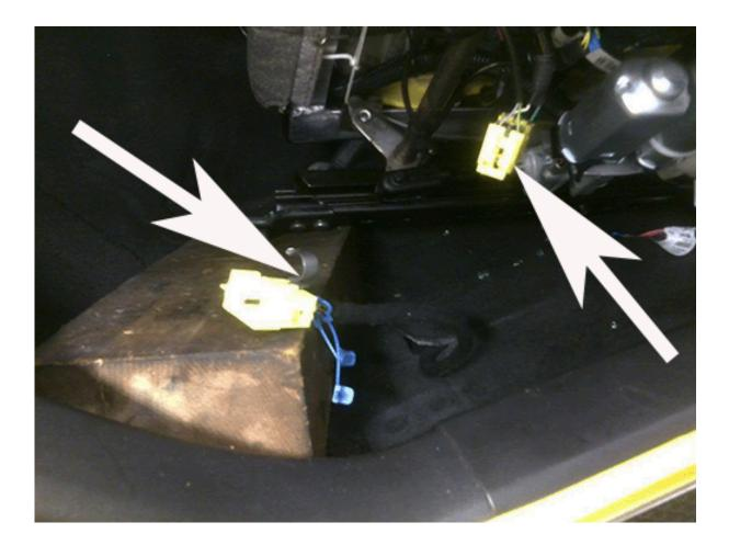
1. Locate the yellow harness connector. Disconnect the seat side connector from the vehicle side connector.
