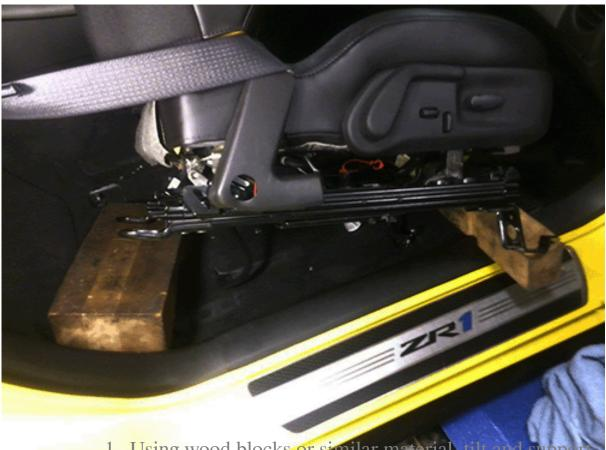
1. Using wood blocks or similar material, till and su the seat in the vehicle as shown.
