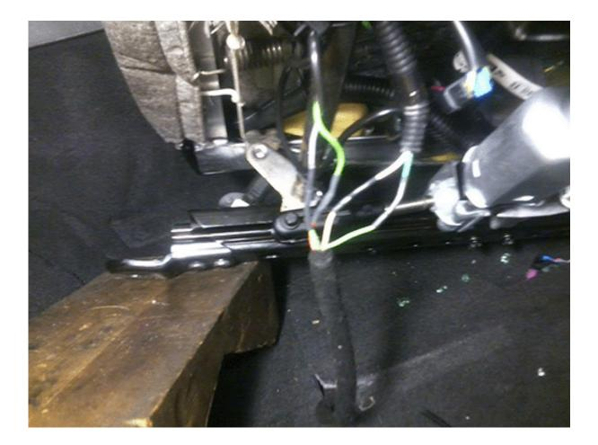
Crimp a splice clip over the joined wires using Special Tool J-38125-8, nest F. Verify the crimp quality. Repeat this crimp process on all four wire connections (2).
