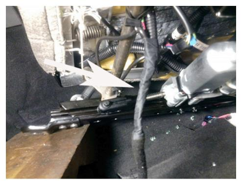
3. Wrap woven polyester electrical tape (PET) or equivalent anti-abrasion tape around the spliced section of seat harness.
