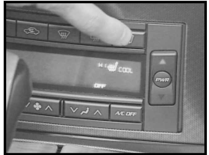
Figure 5-9, Seat Heating/Cooling Controls at HVAC Control Head
