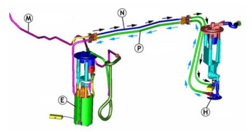
**TIP:** The pressure regulator is in the fuel tank, not on the fuel rail on the engine. This type of fuel system is called returnless, or demand. This means that excess fuel is diverted before it leaves the tank, instead of passing through the fuel rail before being diverted. The result is that hot fuel is not constantly returning from the engine compartment, so the fuel in the tank stays cooler, improving evaporative emissions.
