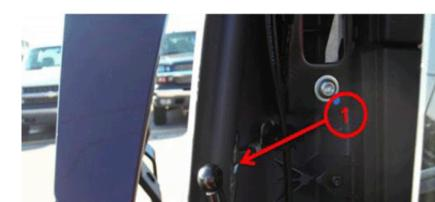
When the adjuster link from the quarter glass hinge is bent, it is outboard. Refer to call out 1 in the illustration above. Bend the link back inboard until it will just touch the inside surface of the weatherstrip. When in the right position it could be forced passed the weather strip with minimal effort.
