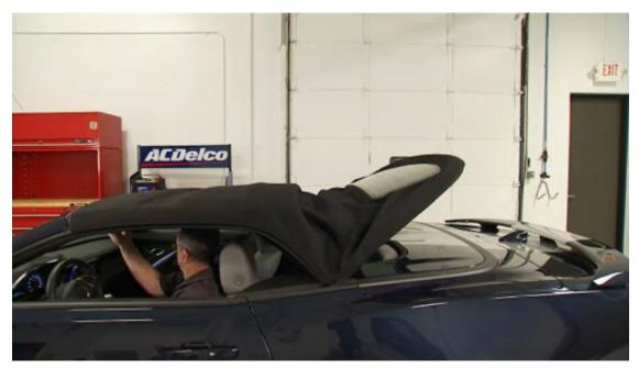
On a correctly working car, the stowage compartment lid must close completely before the tension bow is commanded down. Because the steps or phases must be completed in order, the technician must go to the point where the failure occurs, and then go back one step to look at the scan tool data.
