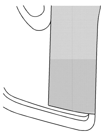
5. Use a pair of scissors to trim off excess foam to the edge of the deck lid inner.
